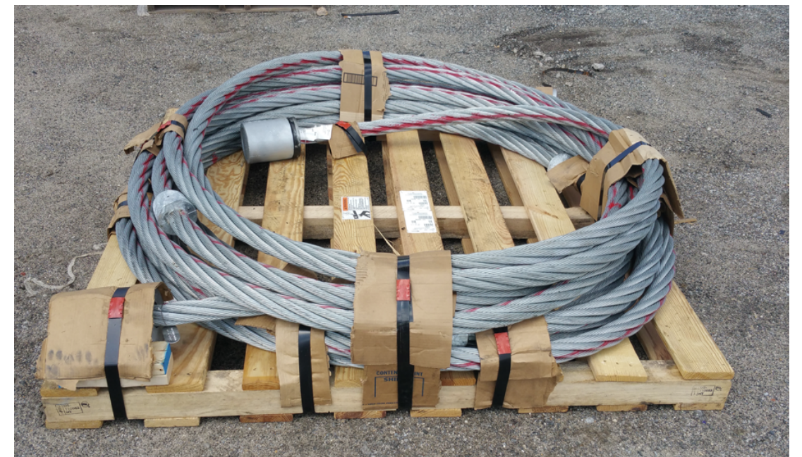
EXAMPLE SUSPENDER ROPE DELIVERED TO PROJECT SITE WITH RED STRIPE
